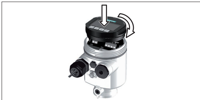
Fig. 16: Insertion of the display and adjustment module with single chamber housing
